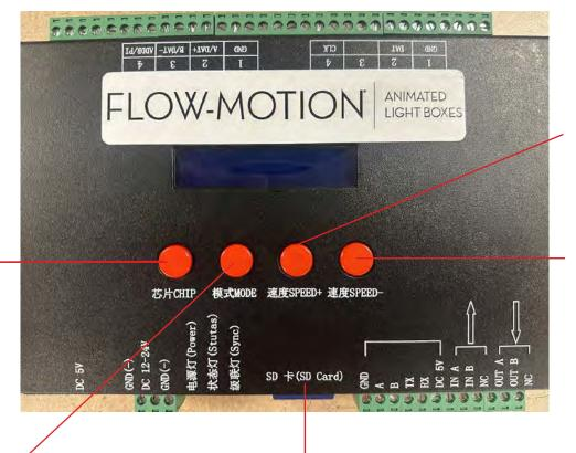
Increase the speed of the program by pressing the "Speed "+" button.
