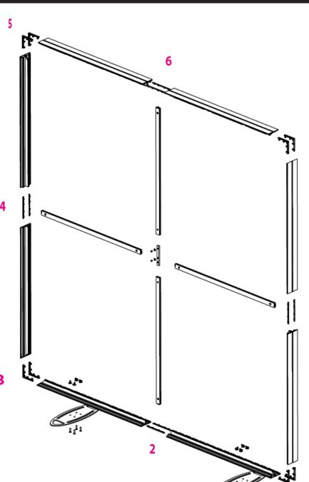
3. ASSEMBLE LONG VERTICAL SUPPORTS BY COUPLING THE 2 SECTIONS USING THE VERTICAL INSERT AND INCLUDED HARDWARE.
