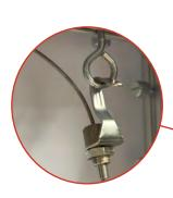
**1.)** Adjust top hooks so they are 3" from the top of the board. Hang the lights in front of the support bars with the open side of the hook and the LEDS are facing out. Next hook the bottom of the light through the eyelet and pull cable to tighten the lights.
