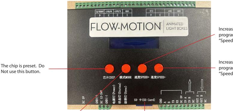
Increase the speed of the program by pressing the "Speed+" button.
