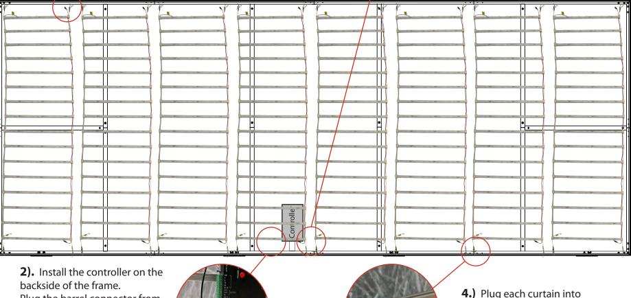
backside of the frame. Plug the barrel connector from the controller and all the light curtains into the into the corresponding power supply.
