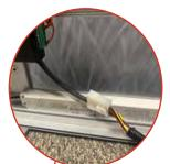
**3).** Layout each wire harness across the bottom of the frame one on the left side and on the right. (NOTE: each is the same and will fit either side) Plug each harness into the controller.
