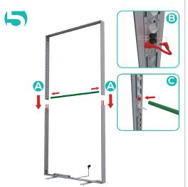
Place the top half of the extrusion and slide onto the split connector of the bottom half extrusion. Connect LED Wire Connector to LED strips. Install Support Pole on each side of the inner frame.
