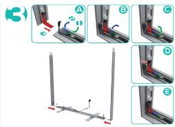
Slide side extrusions into bottom extrusion channel. Use latch to press down on the L connector. Then press down the second latch to secure.
